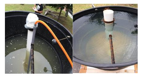
Figure 6 and 5: The clarity of solar pond before and after the particles settle down to the bottom of the pond.
