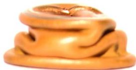
Figure 12 Comparison of deformed tube – (a) quasi-static compression, irregular swelling and (b) ultrasonic compression, regular swelling
