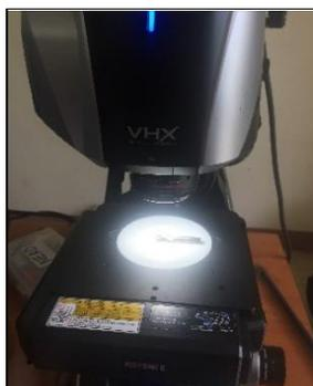
Figure 2: Keyence VHX-6000 digital microscope
