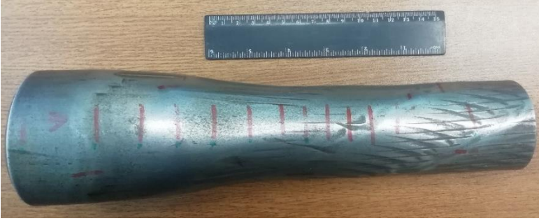
Figure 4: The specimen of the tube for the hardness test
