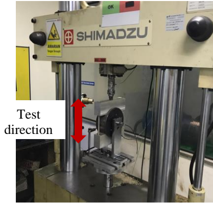
Figure 3: Experimental setup that show the testing machine for assessing the stiffness of the MRE bushing
