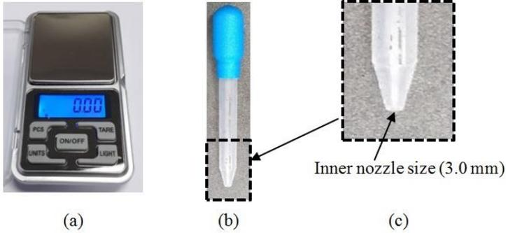
Figure 2: (a) Digital weight measurement, (b) manual droplet dispenser, and (c) inner nozzle size (3.0 mm)
