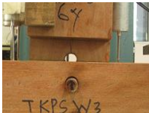
Figure 5: Half of hole can be seen and associated with decreasing load
