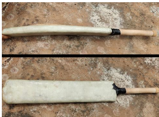
Figure 4: Side view (top) and front view (bottom) of the composite layered cricket bat
