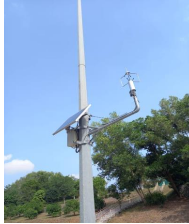
(b) Final installation of ultrasonic anemometer in Precinct 9 (UKM02)
