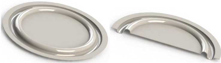
Figure 8: Proposed corrugated configuration for the circular diaphragm and its cross-section.
