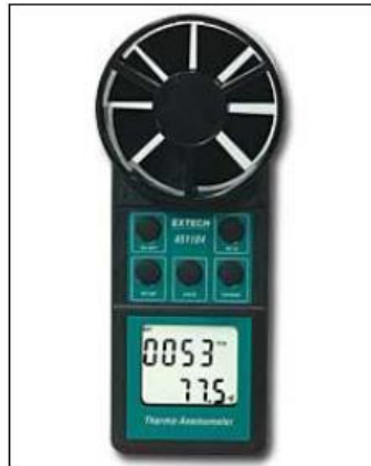
Figure 4: Thermo Anemometer used to record temperature.
