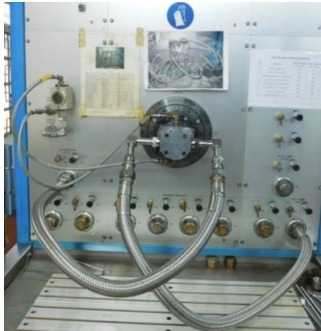
Figure 7: Picture of assembled pump with test rig.
