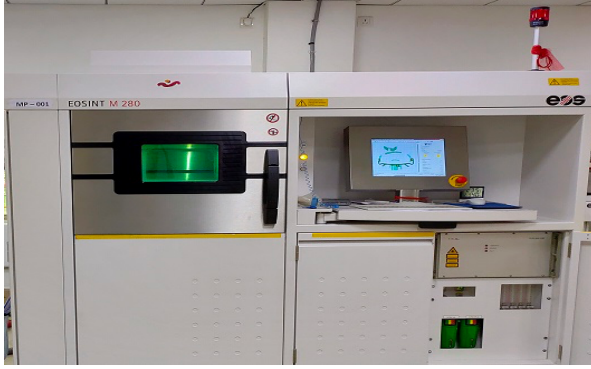
Figure 2: EOSINT M280 DMLS Machine used for manufacturing.
