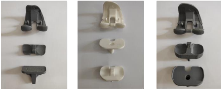
Figure 4: 3D printed of TKR using FDM.
