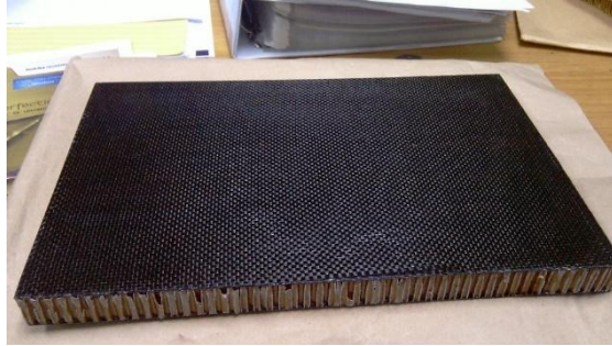
Figure 8: Completed and well cured specimen of honeycomb core sandwich composite panel.
