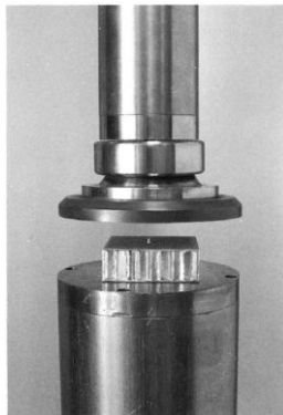
Figure 9: Sandwich panel placed between a set of loading platens in the testing machine [21].
