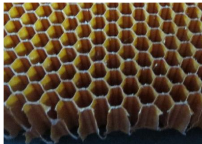
Figure 5: Actual Nomex ®honeycomb used as specimen in the experiment.
