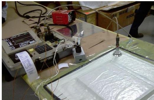
Figure 7: Heatcon ® Hot Bonder system and curing process of honeycomb core sandwich composite panel under vacuum and heat.
