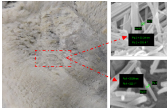
Figure 4: Diameter size of single ANFs under FESEM observation
