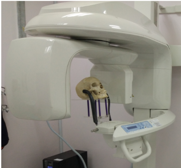
Figure 5: Human skull model set up on platform X-ray desktop.
