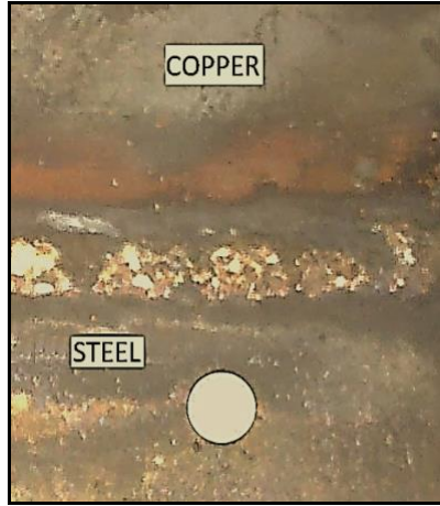
Figure 1: A weld between copper and steel used in parts of a metallurgical crystallizer
