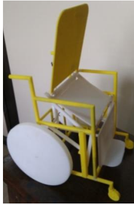
Figure 8: 3D printed prototype with standing configuration
