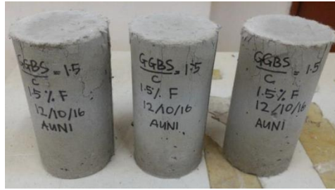
Figure 5: ECC cylinders after compression test.
